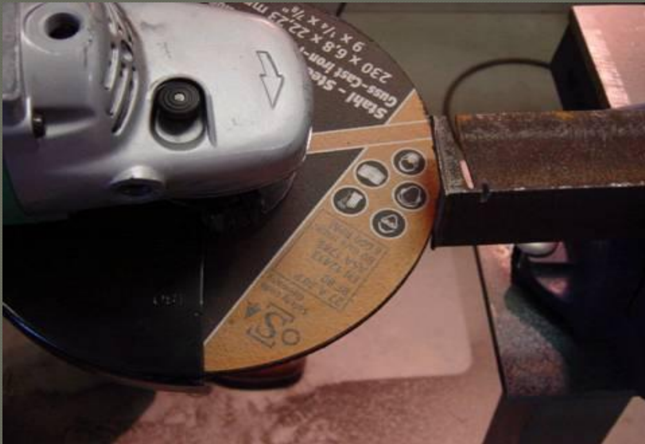
Dressing edge of Grinding Wheel
